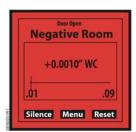
If pressure falls outside of preset limits (Alarmed State), the screen is red
