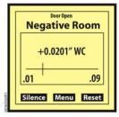
When the door is open, the screen is yellow until the alarm delay is reached
